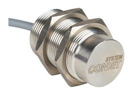
Contrinex inductive proximity sensor, tubular, 30mm diameter x 50mm body, stainless steel housing, PNP, N.O. output, 40mm sensing distance, non-flush, 90 Hz switching frequency, IP68 IP69K, pigtail.
