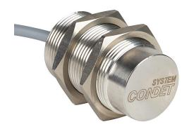
Contrinex inductive proximity sensor, tubular, 30mm diameter x 50mm body, stainless steel housing, PNP, N.O. output, 40mm sensing distance, non-flush, 90 Hz switching frequency, IP68 IP69K, pigtail.
