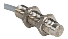
Contrinex inductive proximity sensor, tubular, 12mm diameter x 50mm body, stainless steel housing, PNP, N.O. output, 10mm sensing distance, non-flush, 400 Hz switching frequency, IP68 IP69K, pigtail.
