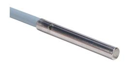
Contrinex inductive proximity sensor, tubular, 4mm diameter x 30mm body, stainless steel housing, PNP, N.O. output, 3mm sensing distance, non-flush, 1.2 kHz switching frequency, IP67, pigtail.
