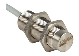
Contrinex inductive proximity sensor, tubular, 18mm diameter x 50mm body, stainless steel housing, NPN, N.C. output, 20mm sensing distance, non-flush, 200 Hz switching frequency, IP68 IP69K, pigtail.
