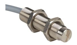
Contrinex inductive proximity sensor, tubular, 12mm diameter x 50mm body, stainless steel housing, NPN, N.C. output, 10mm sensing distance, non-flush, 400 Hz switching frequency, IP68 IP69K, pigtail.
