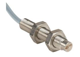
Contrinex inductive proximity sensor, tubular, 8mm diameter x 45mm body, stainless steel housing, NPN, N.O. output, 6mm sensing distance, non-flush, 700 Hz switching frequency, IP67 IP68, pigtail.
