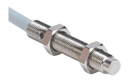
Contrinex inductive proximity sensor, tubular, 5mm diameter x 30mm body, stainless steel housing, NPN, N.O. output, 3mm sensing distance, non-flush, 1.2 kHz switching frequency, IP67, pigtail.
