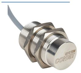
Contrinex inductive proximity sensor, tubular, 30mm diameter x 50mm body, stainless steel housing, NPN, N.O. output, 40mm sensing distance, non-flush, 90 Hz switching frequency, IP68 IP69K, pigtail.
