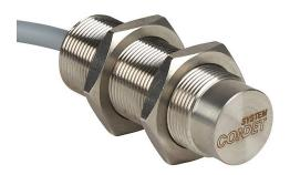
Contrinex inductive proximity sensor, tubular, 18mm diameter x 50mm body, stainless steel housing, NPN, N.O. output, 20mm sensing distance, non-flush, 200 Hz switching frequency, IP68 IP69K, pigtail.
