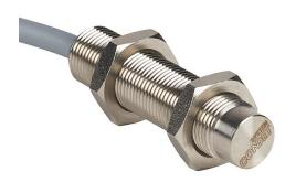
Contrinex inductive proximity sensor, tubular, 12mm diameter x 50mm body, stainless steel housing, NPN, N.O. output, 10mm sensing distance, non-flush, 400 Hz switching frequency, IP68 IP69K, pigtail.
