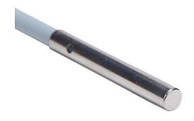
Contrinex inductive proximity sensor, tubular, 4mm diameter x 30mm body, stainless steel housing, NPN, N.O. output, 3mm sensing distance, non-flush, 1.2 kHz switching frequency, IP67, pigtail.
