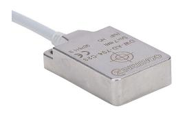
Contrinex inductive proximity sensor, rectangular, 32 x 20 x 8mm body, stainless steel housing, PNP, N.C. output, 7mm sensing distance, flush, 180 Hz switching frequency, IP68 IP69K, pigtail.
