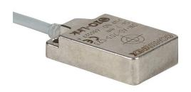
Contrinex inductive proximity sensor, rectangular, 32 x 20 x 8mm body, stainless steel housing, PNP, N.O. output, 7mm sensing distance, flush, 180 Hz switching frequency, IP68 IP69K, pigtail.
