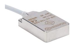
Contrinex inductive proximity sensor, rectangular, 32 x 20 x 8mm body, stainless steel housing, NPN, N.C. output, 7mm sensing distance, flush, 180 Hz switching frequency, IP68 IP69K, pigtail.
