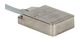
Contrinex inductive proximity sensor, rectangular, 32 x 20 x 8mm body, stainless steel housing, NPN, N.O. output, 7mm sensing distance, flush, 180 Hz switching frequency, IP68 IP69K, pigtail.
