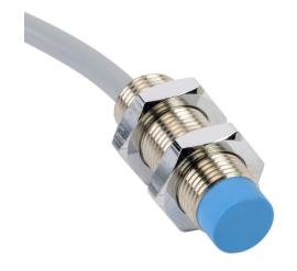
Contrinex inductive proximity sensor, tubular, 12mm diameter x 35mm body, nickel-plated brass housing, PNP, N.O. output, 8mm sensing distance, non-flush, 1.4 kHz switching frequency, IP67, pigtail.
