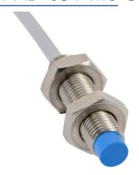
Contrinex inductive proximity sensor, tubular, 8mm diameter x 35mm body, 304 stainless steel housing, NPN, N.O. output, 4mm sensing distance, non-flush, 3.5 kHz switching frequency, IP67, pigtail.
