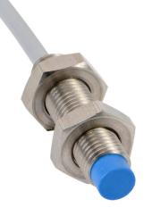
Contrinex inductive proximity sensor, tubular, 8mm diameter x 35mm body, 304 stainless steel housing, NPN, N.O. output, 4mm sensing distance, non-flush, 3.5 kHz switching frequency, IP67, pigtail.
