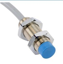
Contrinex inductive proximity sensor, tubular, 12mm diameter x 35mm body, nickel-plated brass housing, NPN, N.O. output, 8mm sensing distance, non-flush, 1.4 kHz switching frequency, IP67, pigtail.
