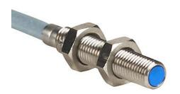
Contrinex inductive proximity sensor, tubular, 4mm diameter x 22mm body, stainless steel housing, PNP, N.C. output, 1mm sensing distance, flush, 3 kHz switching frequency, IP67, pigtail.
