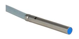
Contrinex inductive proximity sensor, tubular, 3mm diameter x 22mm body, stainless steel housing, PNP, N.C. output, 1mm sensing distance, flush, 3 kHz switching frequency, IP67, pigtail.
