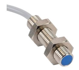
Contrinex inductive proximity sensor, tubular, 8mm diameter x 35mm body, 304 stainless steel housing, PNP, N.O. output, 2mm sensing distance, flush, 5 kHz switching frequency, IP67, pigtail.
