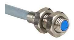
Contrinex inductive proximity sensor, tubular, 4mm diameter x 12mm body, stainless steel housing, PNP, N.O. output, 1mm sensing distance, flush, 8 kHz switching frequency, IP67, pigtail.
