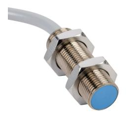
Contrinex inductive proximity sensor, tubular, 12mm diameter x 35mm body, nickel-plated brass housing, PNP, N.O. output, 4mm sensing distance, flush, 2.5 kHz switching frequency, IP67, pigtail.
