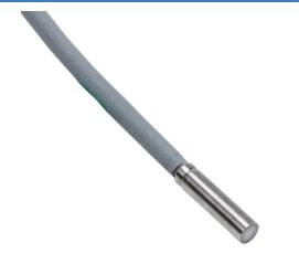
Contrinex inductive proximity sensor, tubular, 3mm diameter x 12mm body, 304 stainless steel housing, PNP, N.O., 0.8mm sensing distance, flush, 8000 Hz switching frequency, IP68 IP69K, pigtail.
