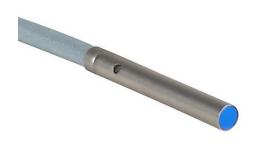
Contrinex inductive proximity sensor, tubular, 3mm diameter x 22mm body, stainless steel housing, NPN, N.C. output, 1mm sensing distance, flush, 3 kHz switching frequency, IP67, pigtail.
