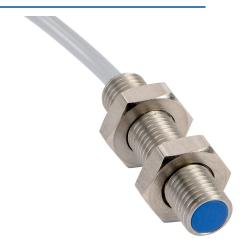
Contrinex inductive proximity sensor, tubular, 8mm diameter x 35mm body, 304 stainless steel housing, NPN, N.O. output, 2mm sensing distance, flush, 5 kHz switching frequency, IP67, pigtail.
