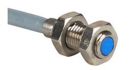
Contrinex inductive proximity sensor, tubular, 4mm diameter x 12mm body, stainless steel housing, NPN, N.O. output, 1mm sensing distance, flush, 8 kHz switching frequency, IP67, pigtail.
