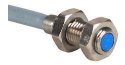
Contrinex inductive proximity sensor, tubular, 4mm diameter x 12mm body, stainless steel housing, NPN, N.O. output, 1mm sensing distance, flush, 8 kHz switching frequency, IP67, pigtail.
