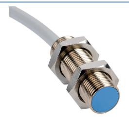
Contrinex inductive proximity sensor, tubular, 12mm diameter x 35mm body, nickel-plated brass housing, NPN, N.O. output, 4mm sensing distance, flush, 2.5 kHz switching frequency, IP67, pigtail.
