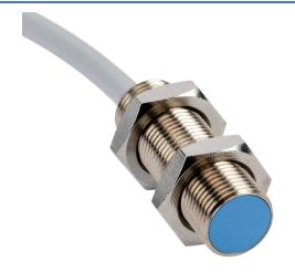
Contrinex inductive proximity sensor, tubular, 12mm diameter x 35mm body, nickel-plated brass housing, NPN, N.O. output, 4mm sensing distance, flush, 2.5 kHz switching frequency, IP67, pigtail.
