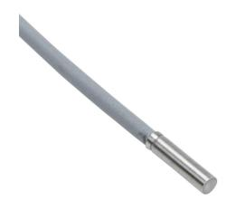
Contrinex inductive proximity sensor, tubular, 3mm diameter x 12mm body, 304 stainless steel housing, NPN, N.O., 0.8mm sensing distance, flush, 8000 Hz switching frequency, IP68 IP69K, pigtail.
