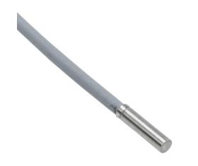
Contrinex inductive proximity sensor, tubular, 3mm diameter x 12mm body, 304 stainless steel housing, NPN, N.O., 0.8mm sensing distance, flush, 8000 Hz switching frequency, IP68 IP69K, pigtail.
