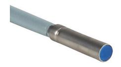
Contrinex inductive proximity sensor, tubular, 3mm diameter x 12mm body, stainless steel housing, NPN, N.O. output, 1mm sensing distance, flush, 8 kHz switching frequency, IP67, pigtail.
