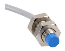
Contrinex inductive proximity sensor, tubular, 8mm diameter x 22mm body, 304 stainless steel housing, PNP, N.O. output, 2.5mm sensing distance, non-flush, 4.5 kHz switching frequency, IP67, pigtail.
