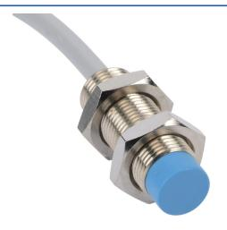
Contrinex inductive proximity sensor, tubular, 12mm diameter x 35mm body, nickel-plated brass housing, PNP, N.O. output, 4mm sensing distance, non-flush, 2 kHz switching frequency, IP67, pigtail.
