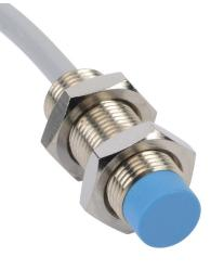
Contrinex inductive proximity sensor, tubular, 12mm diameter x 35mm body, nickel-plated brass housing, PNP, N.O. output, 4mm sensing distance, non-flush, 2 kHz switching frequency, IP67, pigtail.
