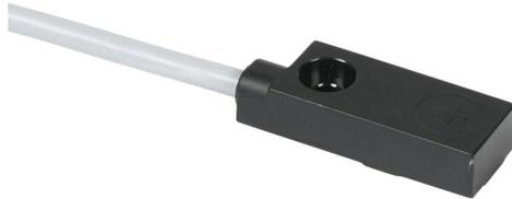
Contrinex inductive proximity sensor, rectangular, 12 x 27 x 6.5mm body, polycarbonate housing, top sensing, PNP, N.O. output, 4mm sensing distance, non-flush, 2000 Hz switching frequency, IP67, pigtail.
