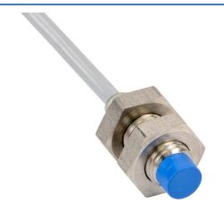
Contrinex inductive proximity sensor, tubular, 8mm diameter x 22mm body, 304 stainless steel housing, NPN, N.O. output, 2.5mm sensing distance, non-flush, 4.5 kHz switching frequency, IP67, pigtail.
