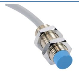
Contrinex inductive proximity sensor, tubular, 12mm diameter x 35mm body, nickel-plated brass housing, NPN, N.O. output, 4mm sensing distance, non-flush, 2 kHz switching frequency, IP67, pigtail.
