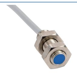
Contrinex inductive proximity sensor, tubular, 8mm diameter x 22mm body, 304 stainless steel housing, PNP, N.O. output, 1.5mm sensing distance, flush, 5 kHz switching frequency, IP67, pigtail.
