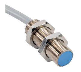
Contrinex inductive proximity sensor, tubular, 12mm diameter x 35mm body, nickel-plated brass housing, PNP, N.O. output, 2mm sensing distance, flush, 3 kHz switching frequency, IP67, pigtail.
