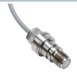
Contrinex inductive proximity sensor, tubular, 10mm diameter x 35mm body, 304 stainless steel housing, PNP, N.O., 0.6mm sensing distance, flush, 2000 Hz switching frequency, IP68, pigtail.
