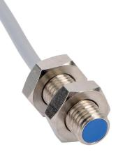
Contrinex inductive proximity sensor, tubular, 8mm diameter x 22mm body, 304 stainless steel housing, NPN, N.O. output, 1.5mm sensing distance, flush, 5 kHz switching frequency, IP67, pigtail.
