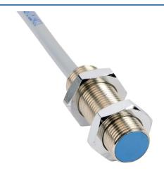
Contrinex inductive proximity sensor, tubular, 12mm diameter x 35mm body, nickel-plated brass housing, NPN, N.O. output, 2mm sensing distance, flush, 3 kHz switching frequency, IP67, pigtail.
