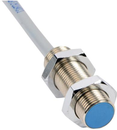
Contrinex inductive proximity sensor, tubular, 12mm diameter x 35mm body, nickel-plated brass housing, NPN, N.O. output, 2mm sensing distance, flush, 3 kHz switching frequency, IP67, pigtail.
