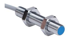
Contrinex inductive proximity sensor, tubular, 8mm diameter x 45mm body, chrome-plated nickel silver housing, PNP, N.C. output, 4mm sensing distance, semi-flush, 500 Hz switching frequency, IP67, pigtail.
