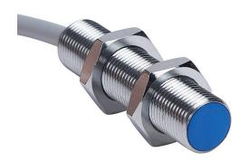
Contrinex inductive proximity sensor, tubular, 12mm diameter x 50mm body, chrome-plated brass housing, PNP, N.C. output, 8mm sensing distance, semi-flush, 400 Hz switching frequency, IP67, pigtail.
