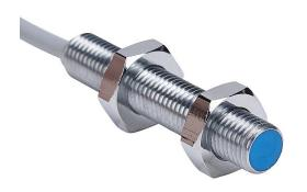
Contrinex inductive proximity sensor, tubular, 8mm diameter x 45mm body, chrome-plated nickel silver housing, PNP, N.O. output, 4mm sensing distance, semi-flush, 500 Hz switching frequency, IP67, pigtail.
