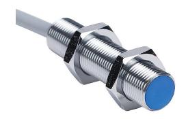
Contrinex inductive proximity sensor, tubular, 12mm diameter x 50mm body, chrome-plated brass housing, PNP, N.O. output, 8mm sensing distance, semi-flush, 400 Hz switching frequency, IP67, pigtail.
