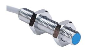
Contrinex inductive proximity sensor, tubular, 8mm diameter x 45mm body, chrome-plated nickel silver housing, NPN, N.O. output, 4mm sensing distance, semi-flush, 500 Hz switching frequency, IP67, pigtail.
