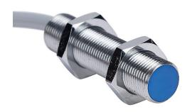
Contrinex inductive proximity sensor, tubular, 12mm diameter x 50mm body, chrome-plated brass housing, NPN, N.O. output, 8mm sensing distance, semi-flush, 400 Hz switching frequency, IP67, pigtail.
