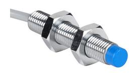
Contrinex inductive proximity sensor, tubular, 8mm diameter x 45mm body, chrome-plated brass housing, PNP, N.C. output, 6mm sensing distance, non-flush, 500 Hz switching frequency, IP67, pigtail.
