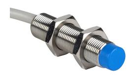
Contrinex inductive proximity sensor, tubular, 12mm diameter x 50mm body, chrome-plated brass housing, PNP, N.C. output, 10mm sensing distance, non-flush, 400 Hz switching frequency, IP67, pigtail.
