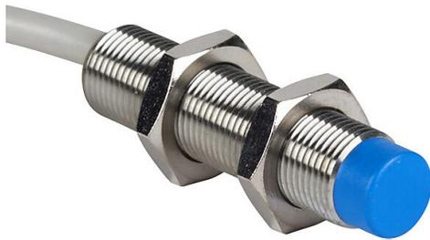
Contrinex inductive proximity sensor, tubular, 12mm diameter x 50mm body, chrome-plated brass housing, PNP, N.C. output, 10mm sensing distance, non-flush, 400 Hz switching frequency, IP67, pigtail.
