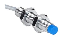
Contrinex inductive proximity sensor, tubular, 8mm diameter x 45mm body, chrome-plated brass housing, PNP, N.O. output, 6mm sensing distance, non-flush, 500 Hz switching frequency, IP67, pigtail.
