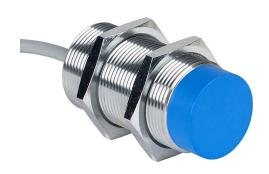
Contrinex inductive proximity sensor, tubular, 30mm diameter x 60mm body, chrome-plated brass housing, PNP, N.O. output, 40mm sensing distance, non-flush, 100 Hz switching frequency, IP67, pigtail.
